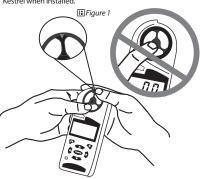
• Orient one "arm" of the module straight up . [1] Figure 2]. The impeller can be pushed in from either side.
