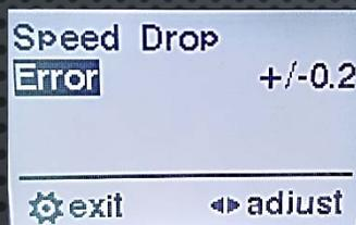
Press the center button to adjust accuracy to either +/- 0.1 or 0.2 mils.
