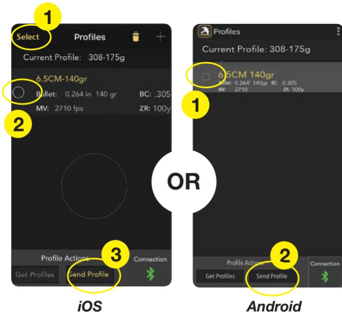
**Note:** You can build and store multiple profiles in the app, but the 2700 can only hold one profile at a time. A profile is any unique combination of gun and bullet. To change profiles, simply transfer a new profile to the 2700.
