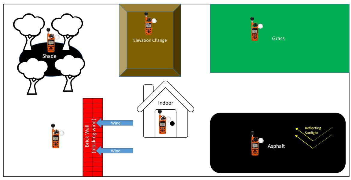
When monitoring WBGT, the Kestrel 5400 should always be placed in the conditions most closely matching those where the people (or animals) are located. Along with temperature and humidity, sun, shade, wind, elevation, and surrounding surfaces all impact the micro-climate and heat stress likelihood, so pay particular attention to matching these conditions.
