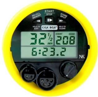
In the CoxBox 08, if your battery cells became unbalanced (where 1 or 2 cells were lower than other), charging to full would result in the fullest cell getting to 100% while the others stayed below 100%). This meant less capacity overall.
