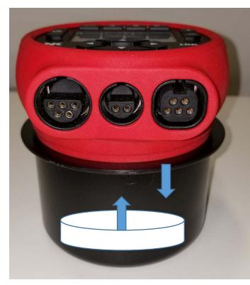
When pressing the CoxBox into the cup holder, it is creating an airtight seal and the result is this air pressure is not allowing the CoxBox to sit at the bottom of the cup.
