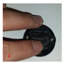
4) Gently press down the battery cover until it snaps into place. Please ensure that the red O-ring is still properly aligned as shown to the left.
