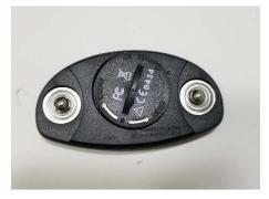
4) Place cover back on. Place nickel or quarter back into center slot. Slightly press down and turn ¼ turn clockwise to seal door back onto buckle.
