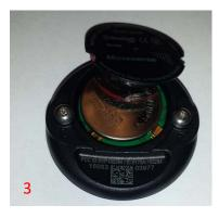
3) Remove the battery cover and then remove the battery. Insert a fresh battery into the same area with label side up.Please note: Battery is a CR2025 model.
