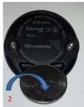
2) Locate a nickel or penny and insert into this indentation so that the coin goes underneath the lip of the battery cover.Press down gently on the edge of the coin to pop open the battery door.
