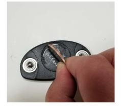
2) Place the nickel or quarter in the middle slot and press down slightly. Turn a ¼ rotation counterclockwise to open.
