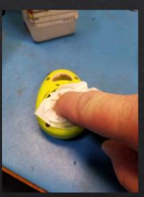
Using a soft cloth or Q-Tip and alcohol gently clean the board under the battery.
