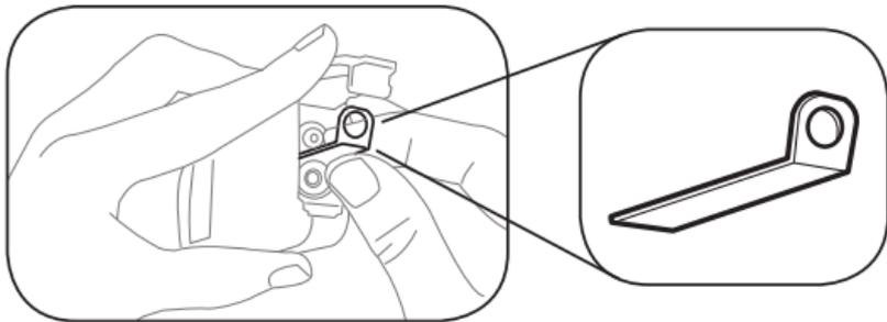
☐ *When replacing batteries in the Kestrel 4500, always keep the shim and re-insert with new batteries as described.*
