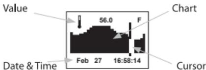
The data value will be displayed at the top of the screen. The date and time when each data point was stored will be displayed at the bottom of the screen.
