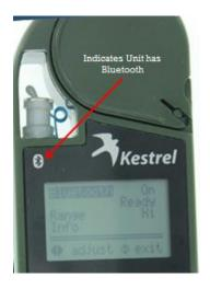
2) Do you have fresh batteries in the Kestrel (Low batteries will display 50% until Bluetooth is turned on, then they will rapidly drain shutting Bluetooth off due to Bluetooth taking a lot of energy)?
